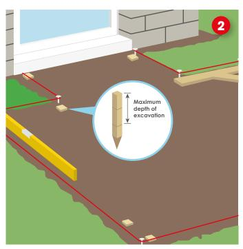
Your patio and any steps must have a gradual slope away from the house to ensure all water drains off. Allow a drop of about 25mm in every 1.5m (diagram 1) or alternatively install a drainage channel. Guidance for installing this should be provided by the drainage channel manufacturer.
